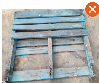
Pallet Boards missing
